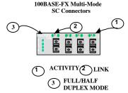
While the functionality of these two modules is essentially the same, the QPM-MSC is equipped with an SC-type "snap-in" connector instead of an ST-type.
